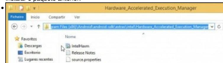
Ir á ruta do SDK /extras/intel/Hardware\_Accelerated\_Execution\_Manager e executar a aplicación IntelHAXM.exe
