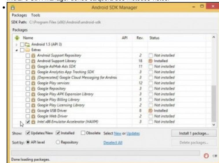
Seleccionar en Extras o paquete Intel Hardware Accelerated Execution Manager. Instalar ...
