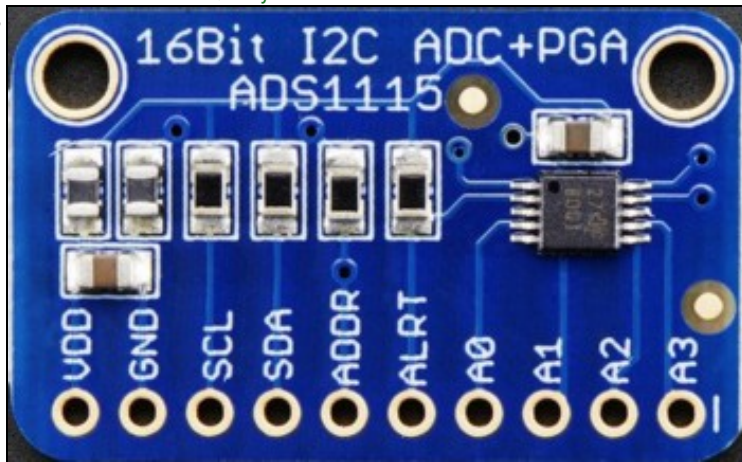
ADS1115 16-Bit ADC - 4 Channel with Programmable Gain Amplifier.
