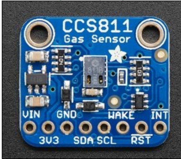
Adafruit CCS811 Air Quality Sensor Breakout - VOC and eCO2.
