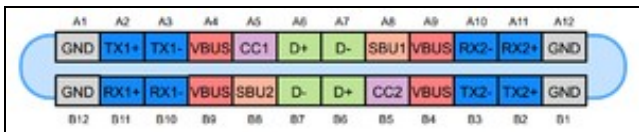
USB Type C pinout
