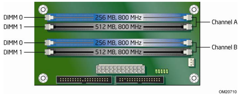
Figure 14. Dual Channel Memory Configuration with Four DIMMs
