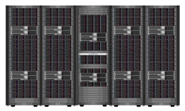
Thus, the result is an external storage system based on HP Scalable File Sharing (HP SFS) Cluster Filesystem of a great scalability and bandwith, with a 219TB raw capacity. The interconnection of the cells to each other and to the calculus system is made through backbone Infiniband. It includes: LINUX operative system, MPI libraries and HP and INTEL mathematics; compilers, purifiers and INTEL optimizers.
