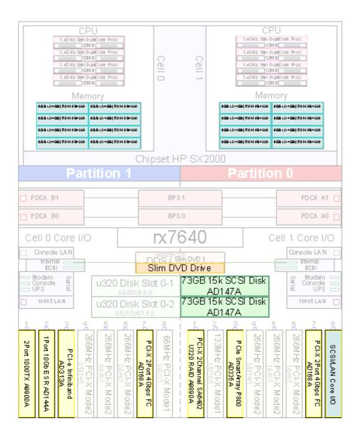
One-cell processors access the local memory of their cell through the 'cell controller' and there exists an interconnection of the different cell controllers that allows each processor to access directly the remote cell memory as well, practically at the same speed, but with a slightly greater latency.
