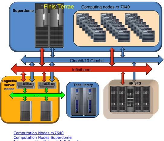
Computation Nodes TX7040 Computation Nodes Superdome Interconnection Network Infiniband HP-SFS storage system Login nodes/file servers Tape library
