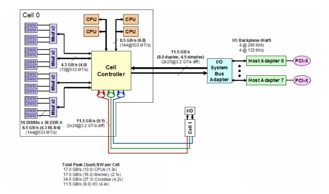
The **architecture** of the system is thus **ccNUMA**: <u>within each computation node, each</u> <u>processor accesses directly to all the memory</u>, although the access time is slightly different depending on whether we are inside the local cell or we are accessing to a remote one. The operative system is in charge of arranging each processor's affinity to its cell's memory, trying to put the data accessed by each processor in their local cell.
