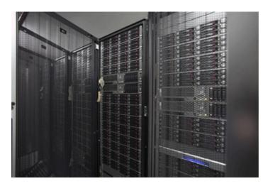
It is a **parallel storage** system, made up of a total amount of 20 servers that have **72 cabins connected to 864 SATA type disks**. The system acts as a great **216 Terabytes** hard disk, shared by all the computation nodes, in a way that the information of this system can be accessed from any of them and at a high speed. *Parallel supercomputing systems need to treat and store great*
