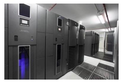
The system has, at the same time, a HP ESL 712e tape library that provides a storage capacity of 2,2 Petabytes of information, in its 1424 slots of type LTO4 tapes. The library has 12 reading units that allow a high transference speed, of almost 3 Gigabytes/seg.
