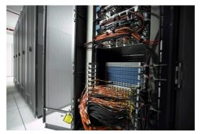
This network has as its most important characteristics the 16 Gbps high interconnection band width, as well as a very low latency, that for the user is 6 microseconds. Each of the computation and storing nodes is connected directly to a great central switch, so every pair of system elements can always communicate at the same speed.
