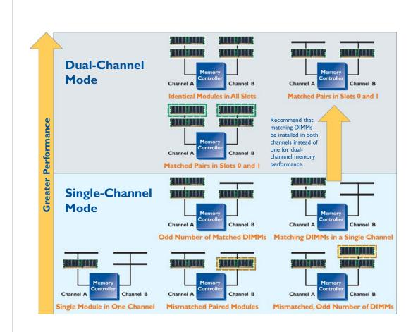
Ideally, with each channel limited to two DIMM sockets, a minimum of two 256MB memory modules should be used for a total memory capacity of 512MB. Only low-end, low-cost systems typically come with a pair of 128MB modules. These 128MB modules are gradually being phased out and will become harder to find as the memory "sweet spot" today is 256MB DIMMs (the "sweet spot" corresponds to the majority of modules shipped in the industry and also offer the best performance to price ratio).
