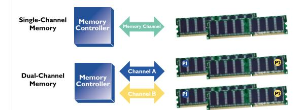
With dual-channel memory, the memory controller is able to move double the peak amount of data that it could normally move with single-channel memory. That's because it is sending or receiving data from two memory module pairs at the same time (shown as module pairs "P1" and "P2" in the graphic above).
