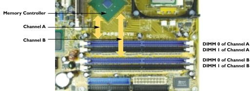
DIMM 0 of Channel A DIMM | of Channel A DIMM 0 of Channel B
