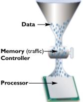
Dual-channel memory utilizes two funnels (and thus two pipes) to feed data to the processor, thereby being able to deliver up to twice the data of the single funnel. With two funnels or channels, data is transferred 128 bits at a time. The process works the
